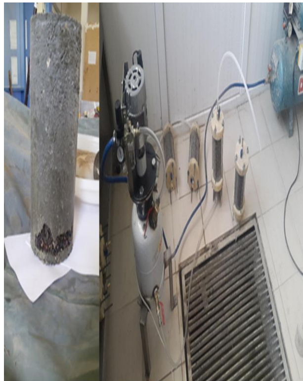
Fig.3- Injection procedure and producing the samples
