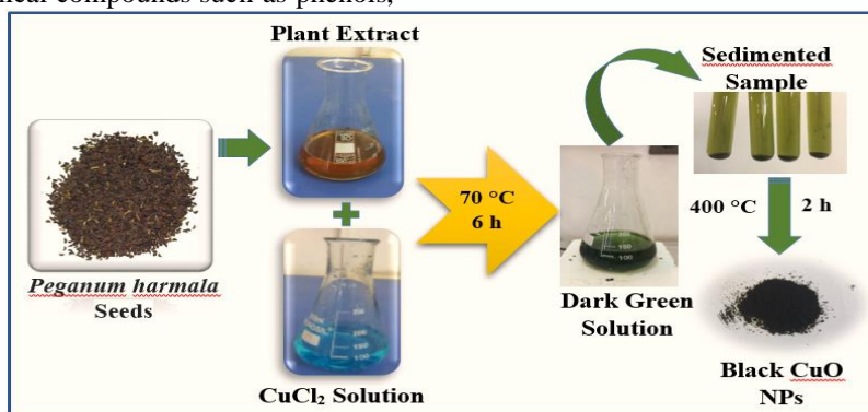
Fig. 1: Schematic overview of the synthesis of CuO NPs using Peganum harmala extract
